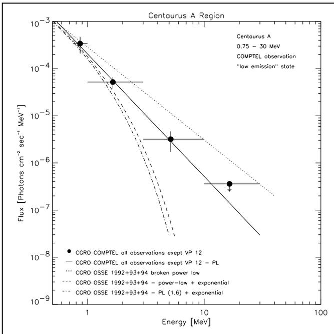
**Fig. 4.** COMPTEL "low state" data with a power-law fit (solid line), the high energy part of the OSSE broken power-law model (dotted line), the OSSE power-law model with an exponential cut-off (dashed line) and the same with a fixed power-law index of  $\alpha = 1.6$  (dash-dot line). See text for more details.
