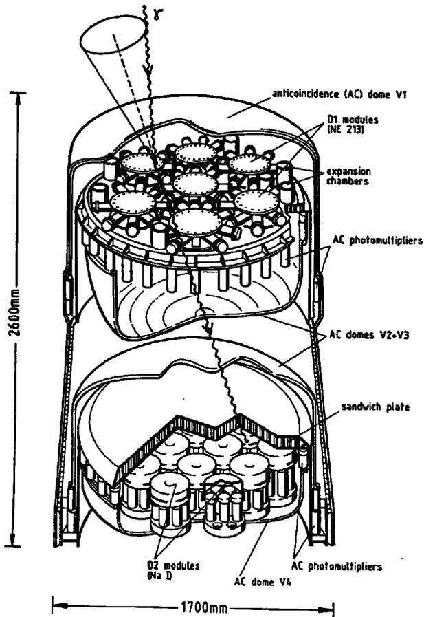
Fig. 1. Schematic drawing of COMPTEL.
